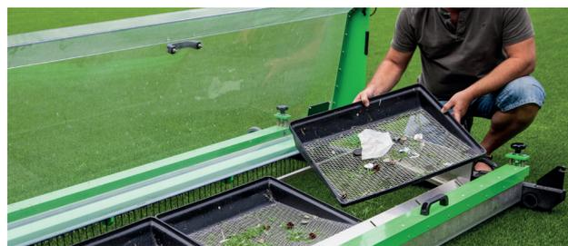
Rubbish and particles that are left in the collection bucket must be removed regularly in order to prevent it from becoming blocked. If the machine is used in rain or wet conditions, the rubber granules will stick to the machine tool and the effect will be reduced.
