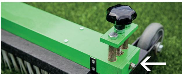
Loosen the lock nut (13 mm) on the ends of the bed cross a couple of turns. The black knob can then be adjusted to the tool having the desired height. Use a 13 mm wrench.
